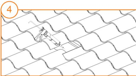
4 Backfill both pilot holes with sealant.
