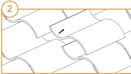
2 Remove the tile where you are installing the hook by gently pulling and pushing the tile.
