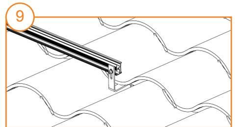
9 Tighten the M8\*25 bolt to secure the rail to the hook.
