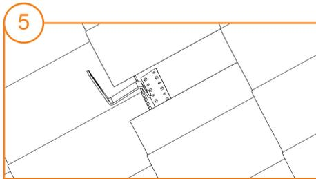
5 Place the hook on top of the rafter to which it will be installed. Make sure the hook is in contact with the tile below it to prevent damage to the roof.
