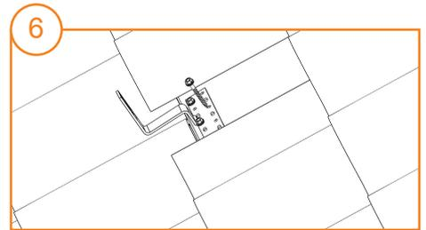
6 Drive three 3/8"/M6.3 bolts into the rafter to secure the hook in place.
