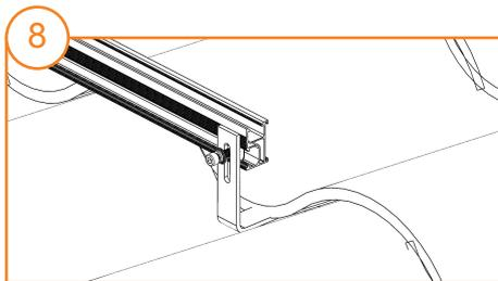
8 Loosely install a M8\*25 inner hex bolt and a rail nut to the hook, then tilt the nut into rail groove.
